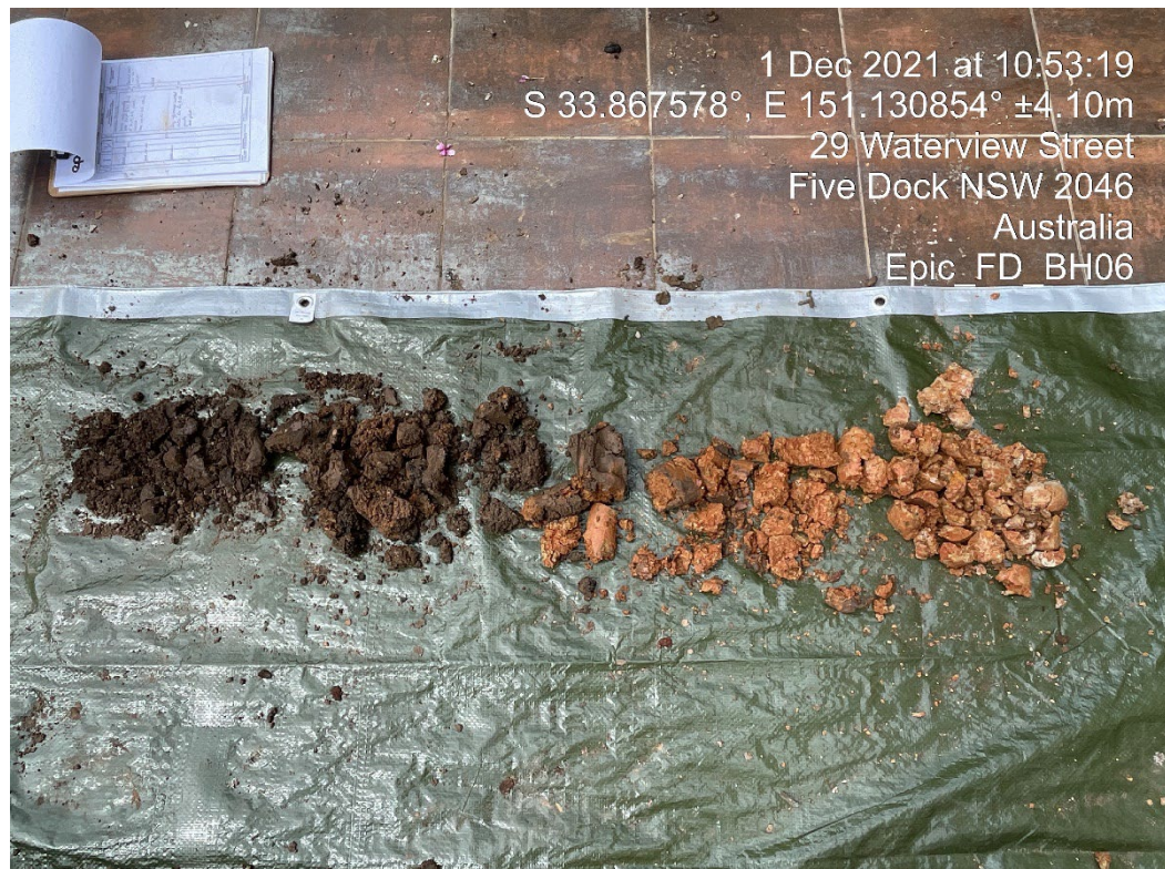
Plate P7: Recovered material at BH06, fill overlying natural clays
