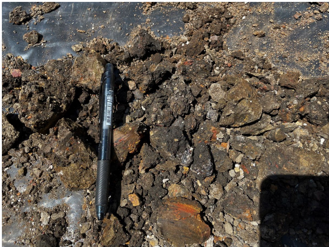
Plate P8: Fill material at BH26
