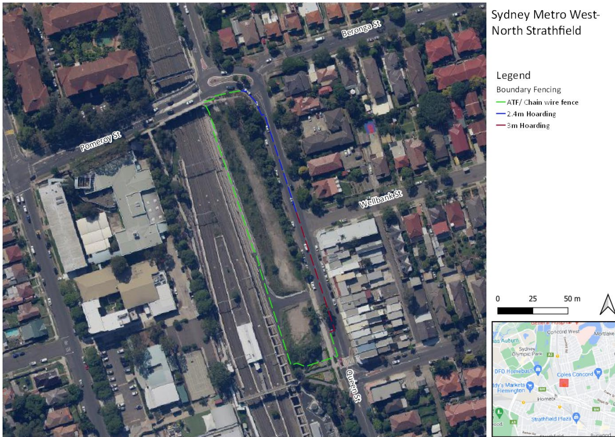
Figure 5-1 North Strathfield Hoarding Layout
