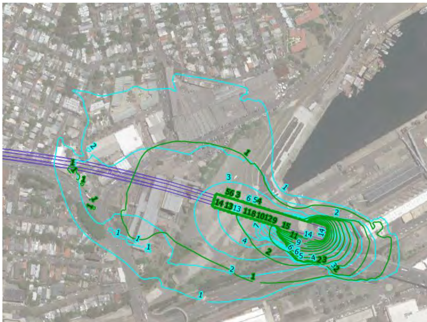
FIGURE 6-16: PREDICTED WATERTABLE DRAWDOWN (METRES) IN MARCH 2023 FOR BASECASE (MITIGATED STATION BOX (1 LUGEON) AND MITIGATED WBPS WITH TUNNELLING SCENARIO) (BLUE) AND UNCERTAINTY SCENARIO WITH SANDSTONE HORIZONTAL HYDRAULIC CONDUCTIVITY EQUAL TO 2.4 LUGEONS (GREEN)
