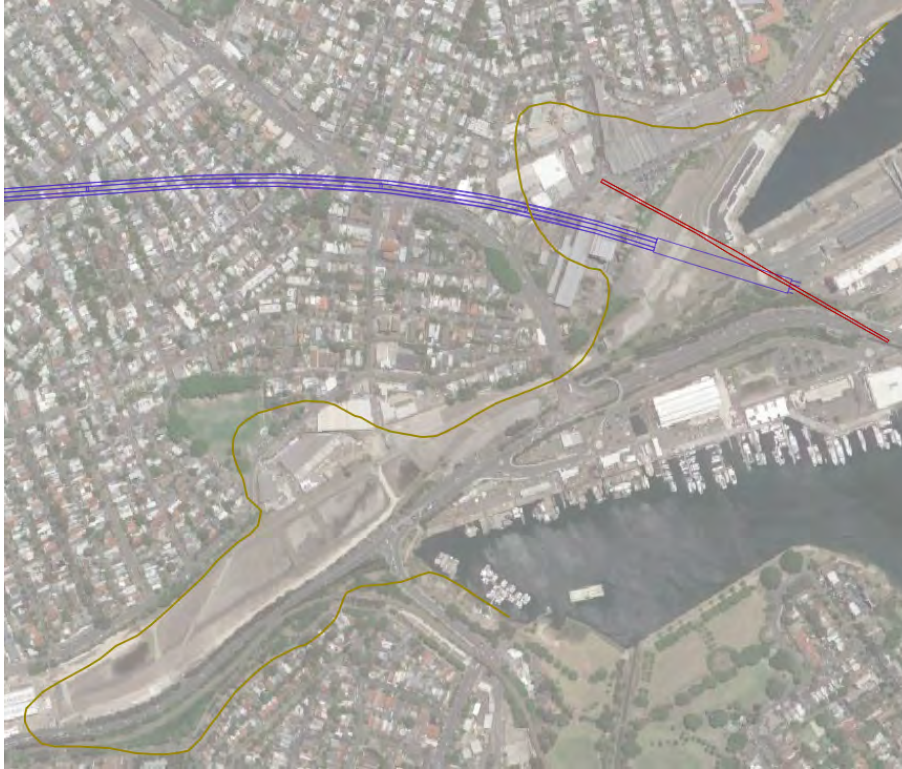
Figure 2.1: Location of the alluvium and Great Sydney Dyke in the vicinity of The Bays Station (Great Sydney Dyke in red, alluvial boundary in orange, station and tunnel alignment in purple).
