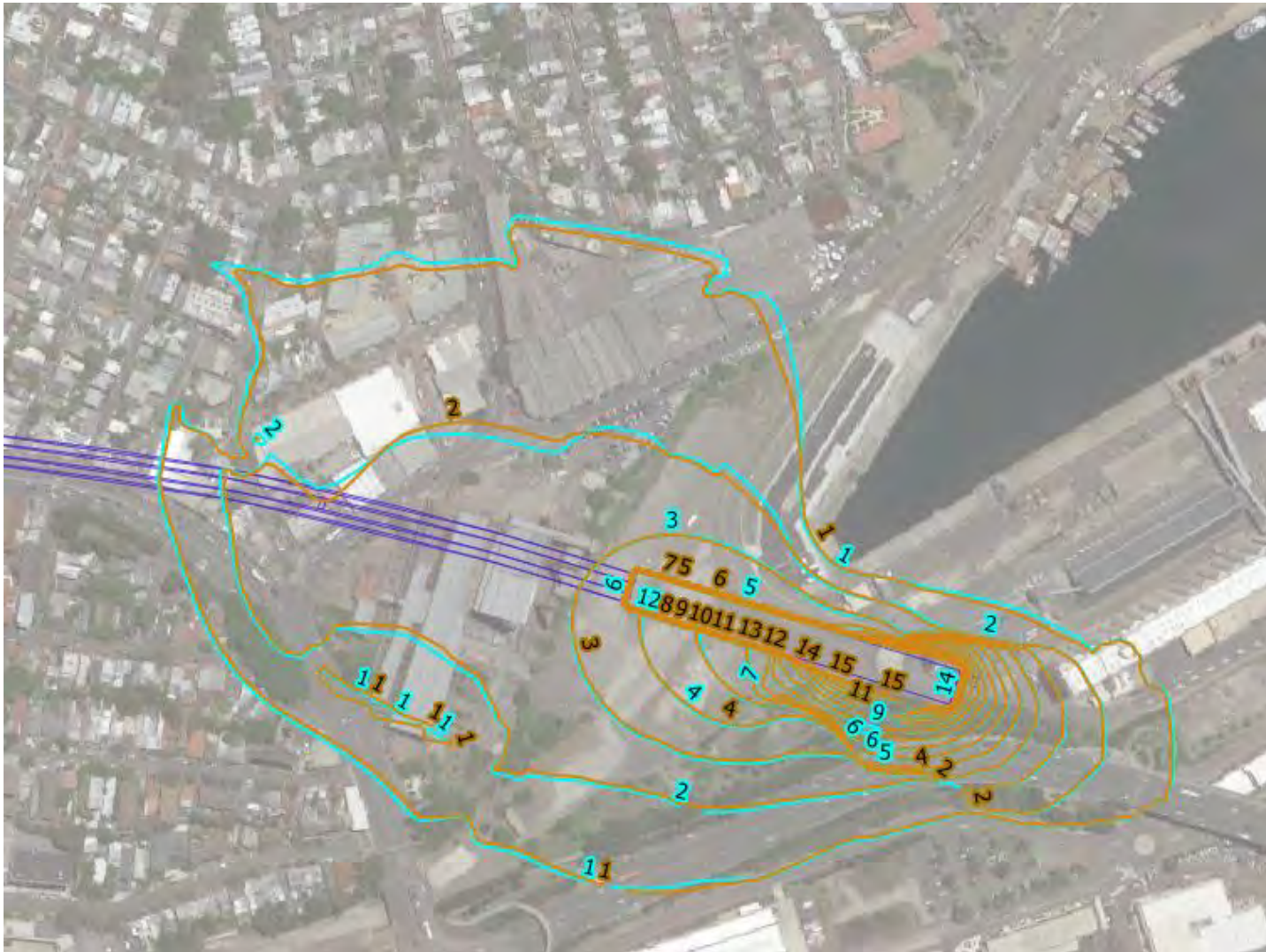
FIGURE 6-15: PREDICTED WATERTABLE DRAWDOWN (METRES) IN MARCH 2023 FOR BASECASE (MITIGATED STATION BOX (1 LUGEON) AND MITIGATED WBPS WITH TUNNELLING SCENARIO) (BLUE) AND UNCERTAINTY SCENARIO WITH ALLUVIUM K_v/K_h = 0.5 (BROWN)
