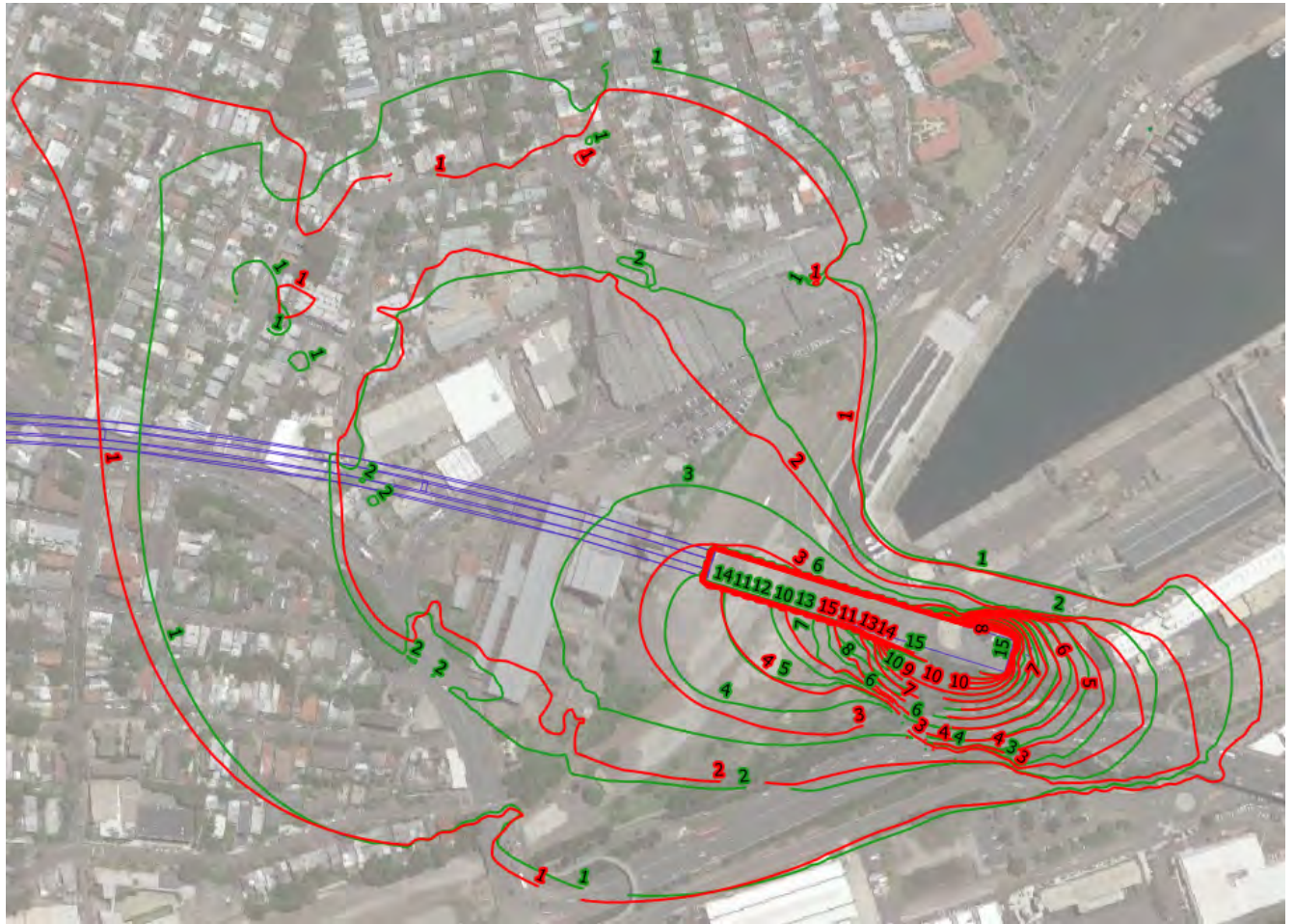
Figure 6.6: Predicted watertable drawdown (m) in Dec 2024 for "Mitigated station box (1 Lugeon) unmitigated WBPS (20 Lugeon rock mass) and CHBC" (green) and "Mitigated station box (1 Lugeon), unmitigated WBPS (80 Lugeons rock mass) and CHBC" scenario (red)
