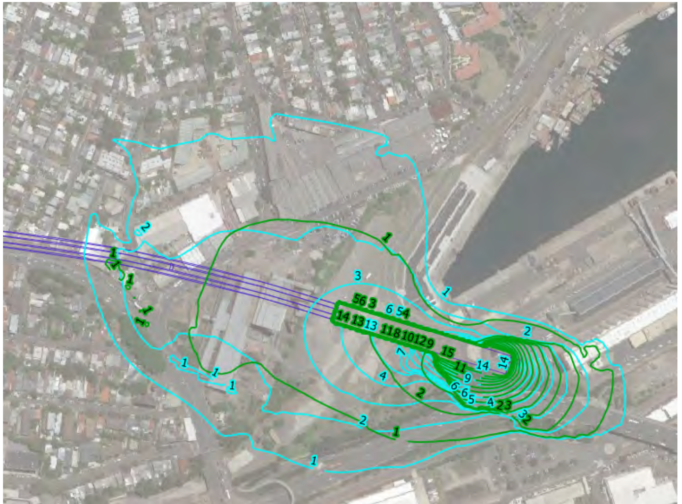
Figure 7.5: Predicted watertable drawdown (metres) in March 2023 for basecase (Mitigated station box (1 Lugeon) and mitigated WBPS with tunnelling scenario) (blue) and sensitivity scenario with sandstone horizontal hydraulic conductivity equal to 2.4 Lugeons (green)
