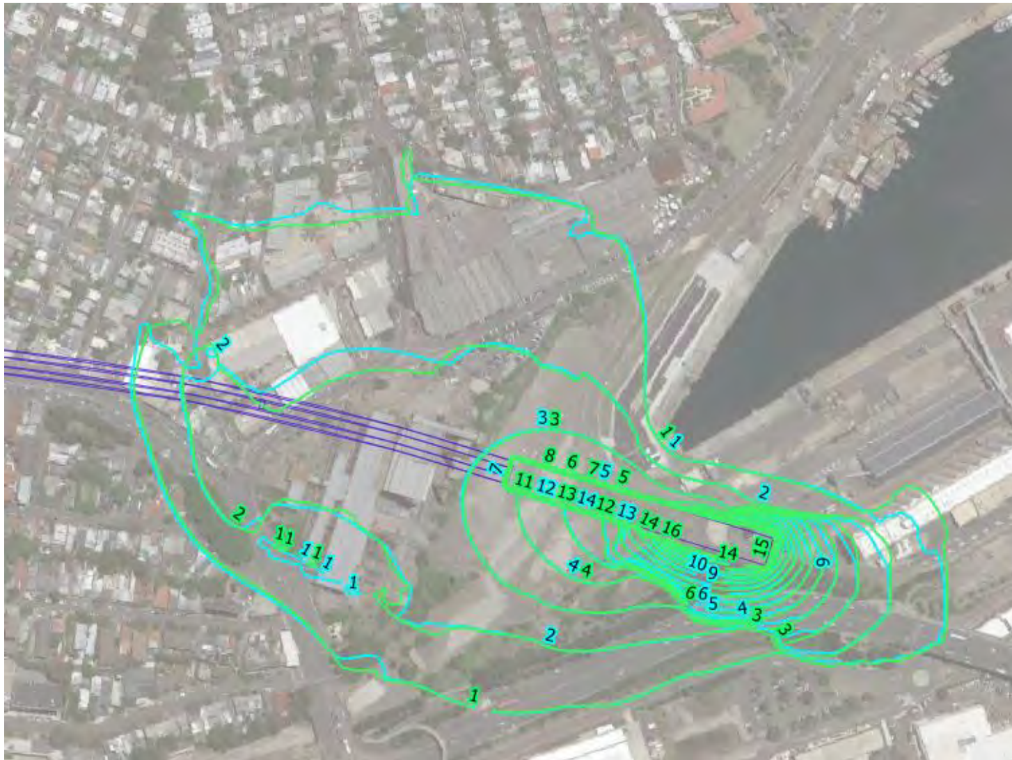
FIGURE 6-14: PREDICTED WATERTABLE DRAWDOWN (METRES) IN MARCH 2023 FOR THE BASE CASE (MITIGATED STATION BOX (1 LUGEON) AND MITIGATED WBPS WITH TUNNELLING SCENARIO) (BLUE) AND UNCERTAINTY SCENARIO WITH RECHARGE OF 1% (GREEN)
