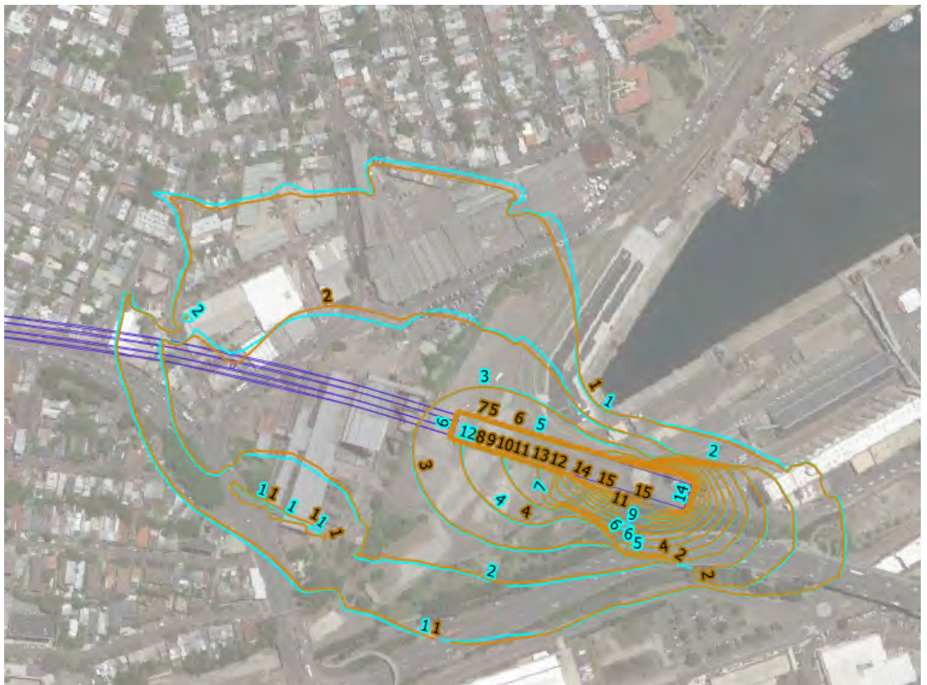
Figure 7.2: Predicted watertable drawdown (metres) in March 2023 for basecase (Mitigated station box (1 Lugeon) and mitigated WBPS with tunnelling scenario) (blue) and sensitivity scenario with alluvium K_v/K_h = 0.5 (brown)
