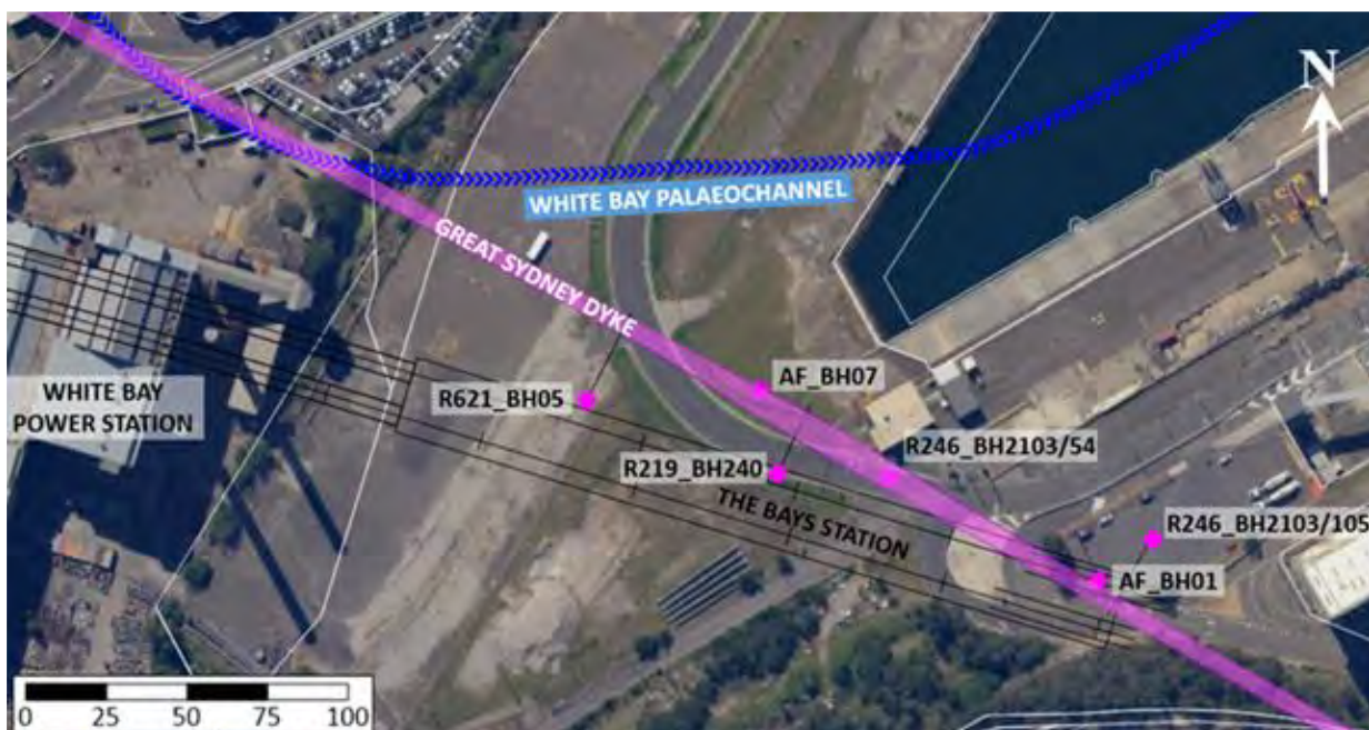
FIGURE 3-8: LOCATION OF BOREHOLES INTERSECTING GREAT SYDNEY DYKE AT THE BAYS STATION SITE
