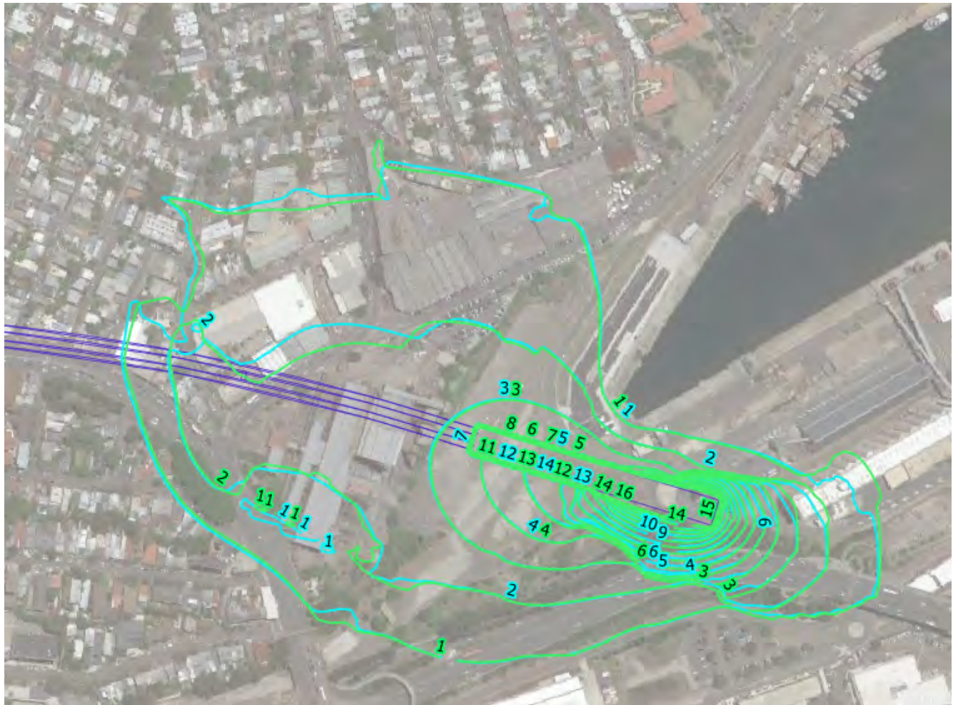
Figure 7.3: Predicted watertable drawdown (metres) in March 2023 for the basecase (Mitigated station box (1 Lugeon) and mitigated WBPS with tunnelling scenario) (blue) and sensitivity scenario with recharge of 1% (green)
