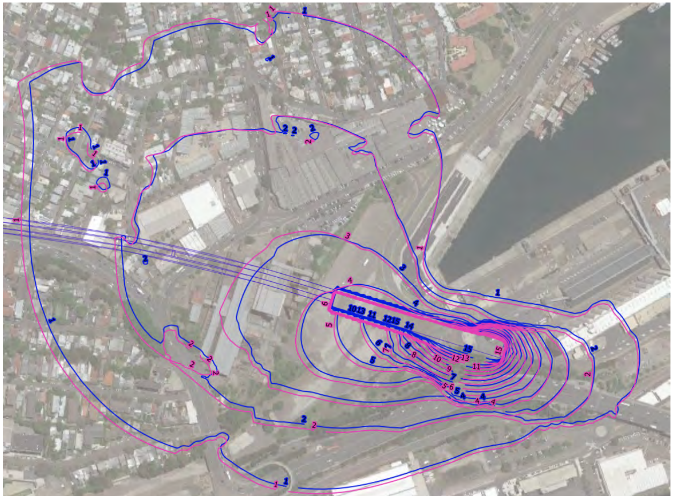
Figure 6.5: Predicted watertable drawdown (m) in December 2024 for "Mitigated station box (1 Lugeon) and mitigated WBPS with tunnelling" scenario (blue) and "Mitigated station box (1 Lugeon) and unmitigated WBPS with tunnelling scenario" (purple)
