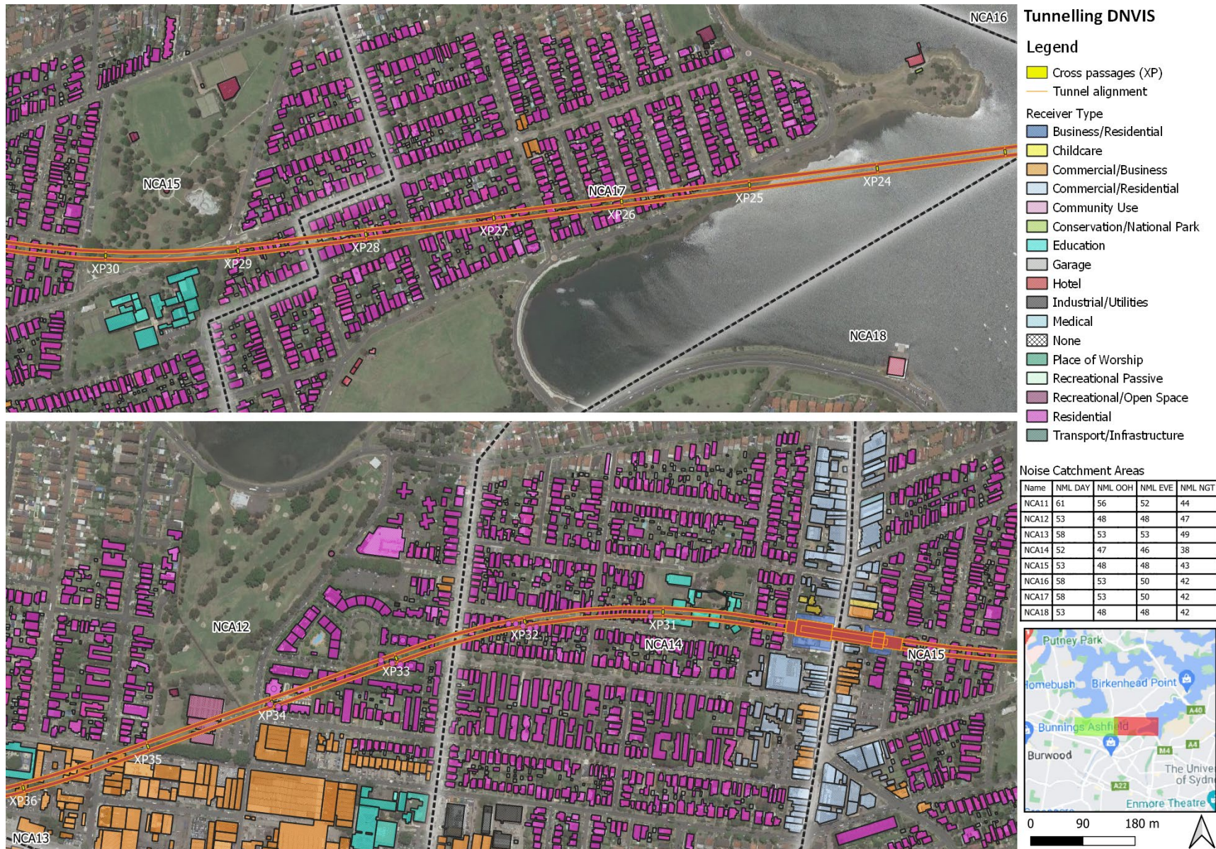
Figure 3-4 Tunnel alignment and sensitive receivers (Five Dock)
