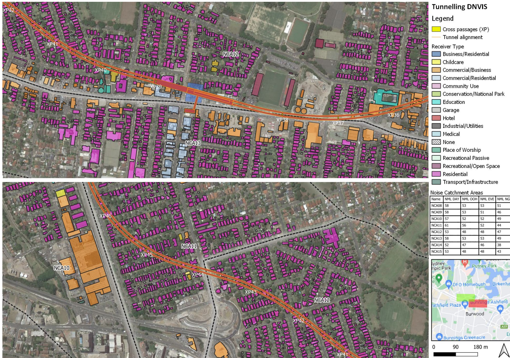
Figure 3-3 Tunnel alignment and sensitive receivers (Burwood North)
